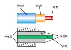
Figure 1 Basic structure of double clad fiber
